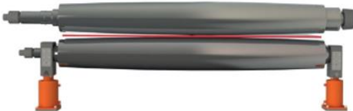
Bending thickness is thinner than roll crowning
