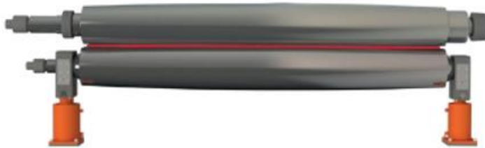
Bending thickness is compatible with roll crowning
