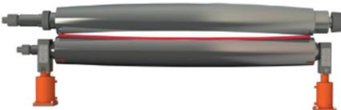
Bending thickness is thicker than roll crowning
