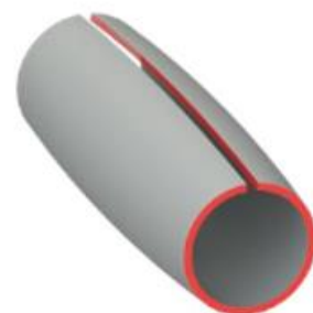
Barrel crowning deformation
