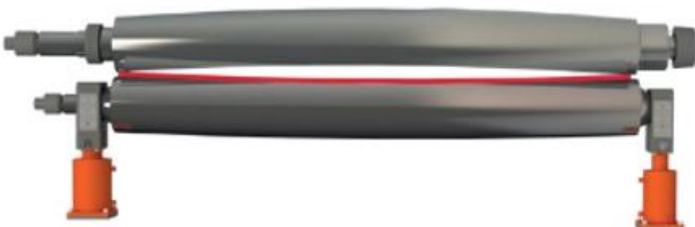
Bending thickness is thicker than roll crowning
