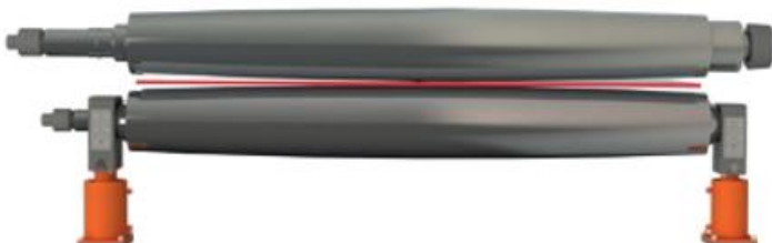
Bending thickness is thinner than roll crowning
